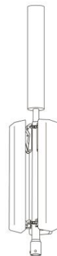
Cylindrical-style antenna atop panel-style antenna(s): cylinder 24 to 50 inches high, 2 to 10 inches in diameter; each panel 24 to 58 inches high, 8 to 12 inches wide, 4 to 10 inches deep, up to 3 panels per pole
