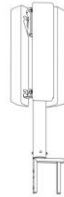
Panel-style antenna(s) each 24 to 58 inches high, 8 to 12 inches wide, 4 to 10 inches deep, Up to 3 panels per pole
