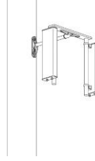
Panel-style antenna(s) each panel 24 to 36 inches high, 8 to 12 inches wide, 6 to 10 inches deep, Up to 3 panels per pole
