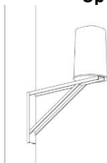
Drum-style antenna 24 to 26 inches high, 16 to 20 inches in diameter
