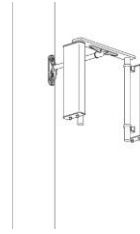
Panel-style antenna(s) each panel 24 to 36 inches high, 8 to 12 inches wide, 6 to 10 inches deep, Up to 3 panels per pole
