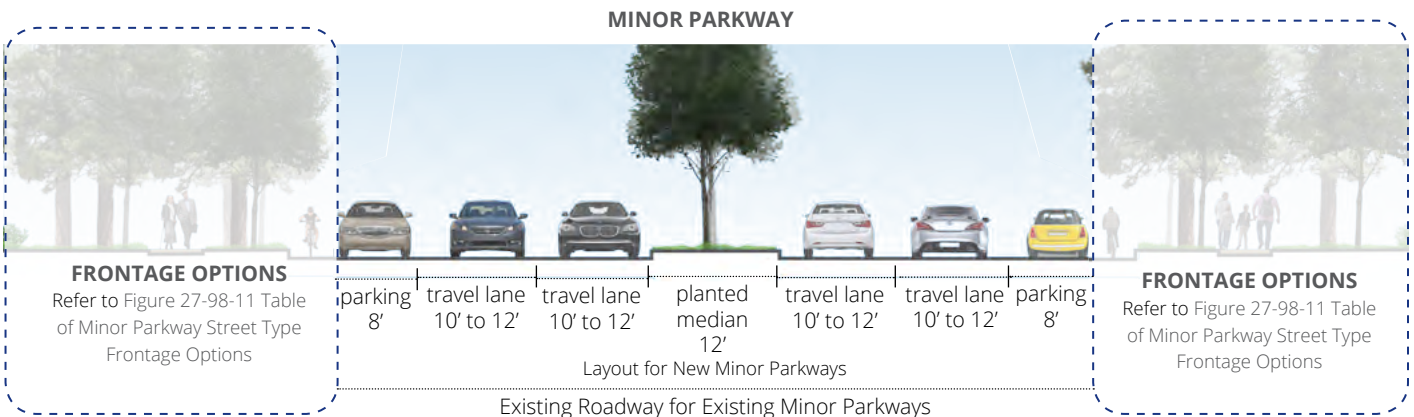
Figure 27-98-10 Minor Parkway Street Section - Existing and New
