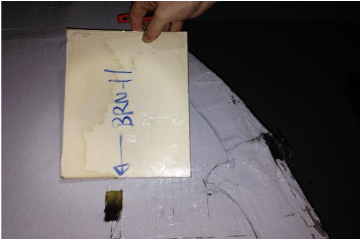
Plate 11: Laboratory analyses did not detect asbestos minerals within HVAC insulation sample BRN-11 collected from the North Administrative Building mechanical room.
