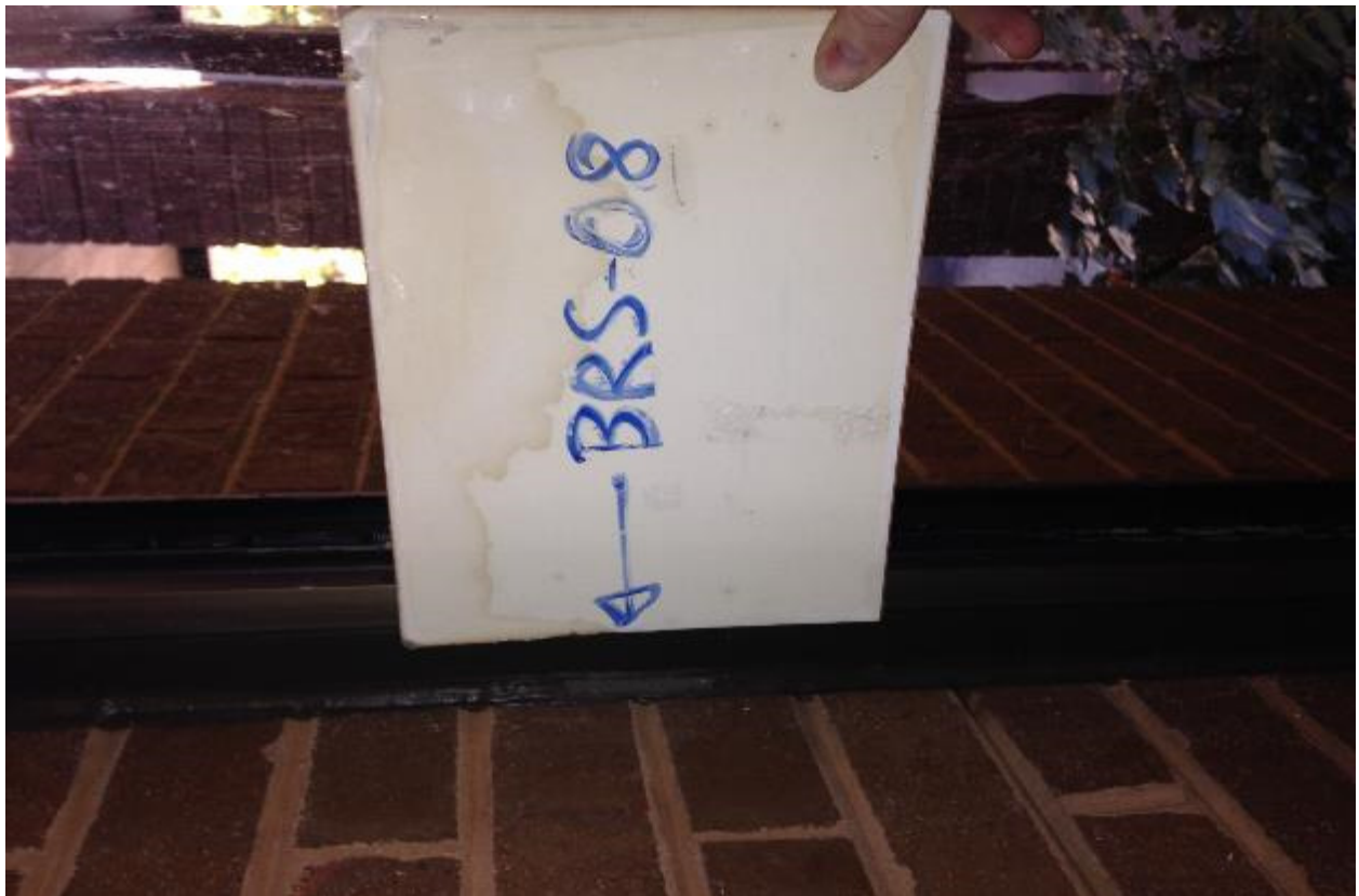
Plate 8: Laboratory analyses did not detect asbestos minerals within the window caulk sample BRS-08 collected from the South Administrative Building windows.
