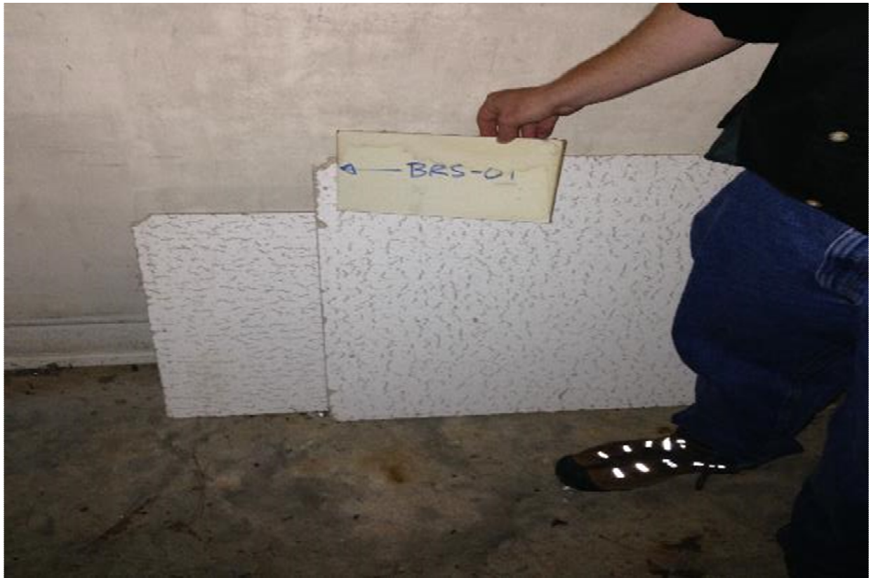
Plate 1: Laboratory analyses did not detect asbestos minerals within suspended ceiling tile sample BRS-01 collected from the South Administrative Building west room.
