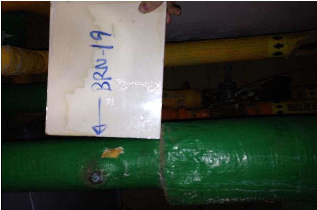
Plate 19: Laboratory analyses did not detect asbestos minerals within plumbing insulation sample BRN-19 collected from the North Administrative Building mechanical room.
