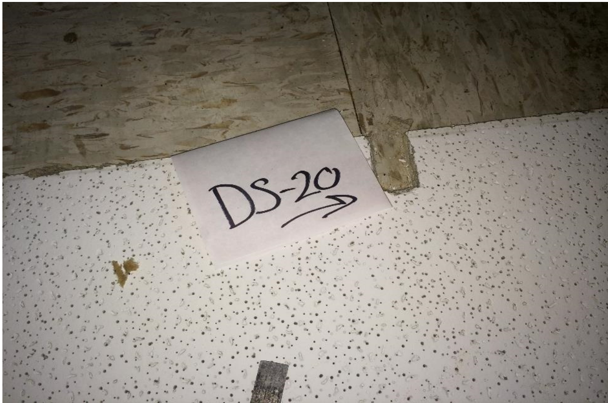
Plate 45: Laboratory analyses did not detect asbestos minerals within suspended ceiling tile sample DS-20 collected from the Dormitory Building downstairs hallways.
