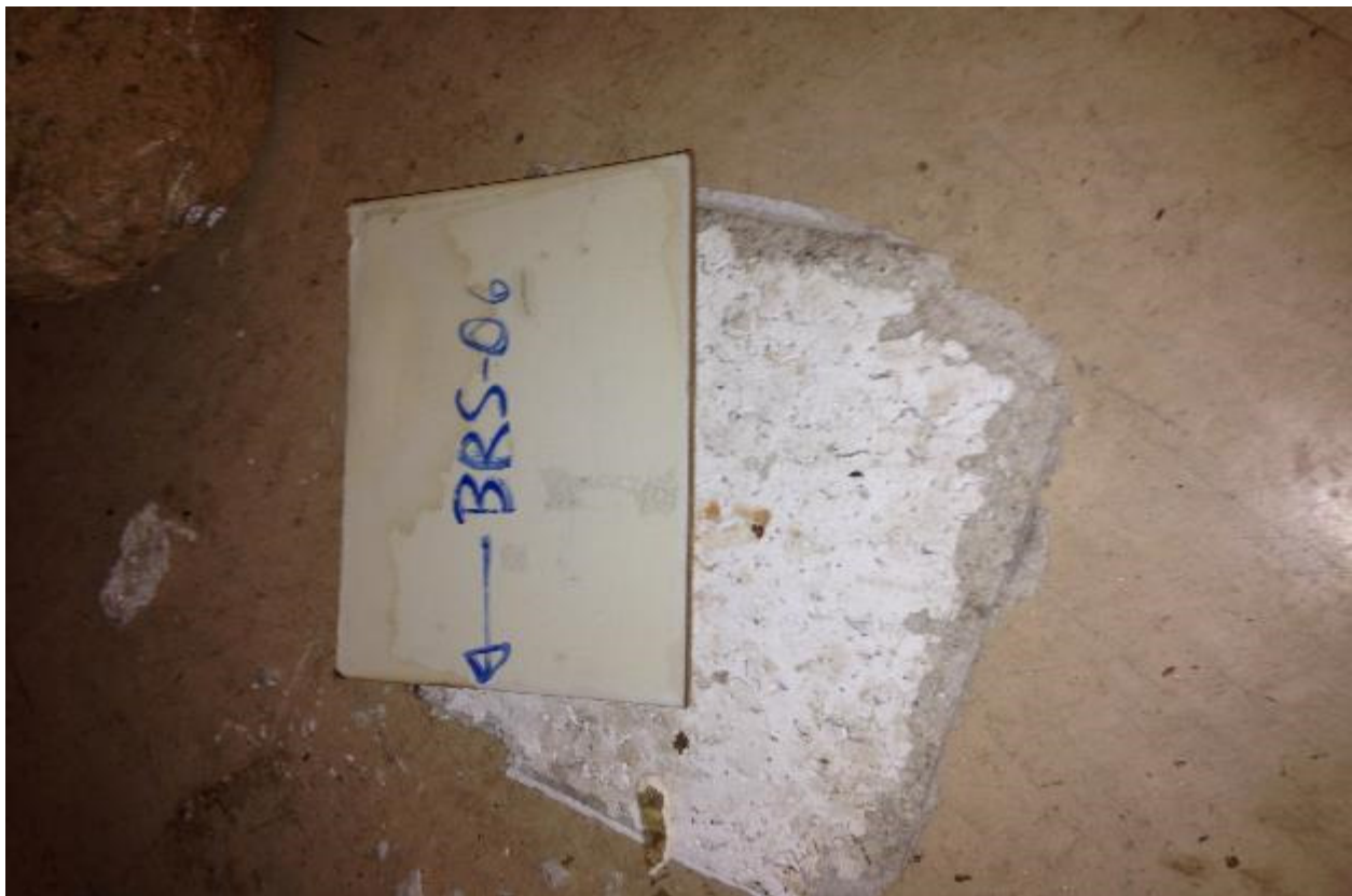
Plate 6: Laboratory analyses detected 2% chrysotile asbestos and 2% amosite asbestos within suspended ceiling tile sample BRS-06 collected from the South Administrative Building east rooms.
