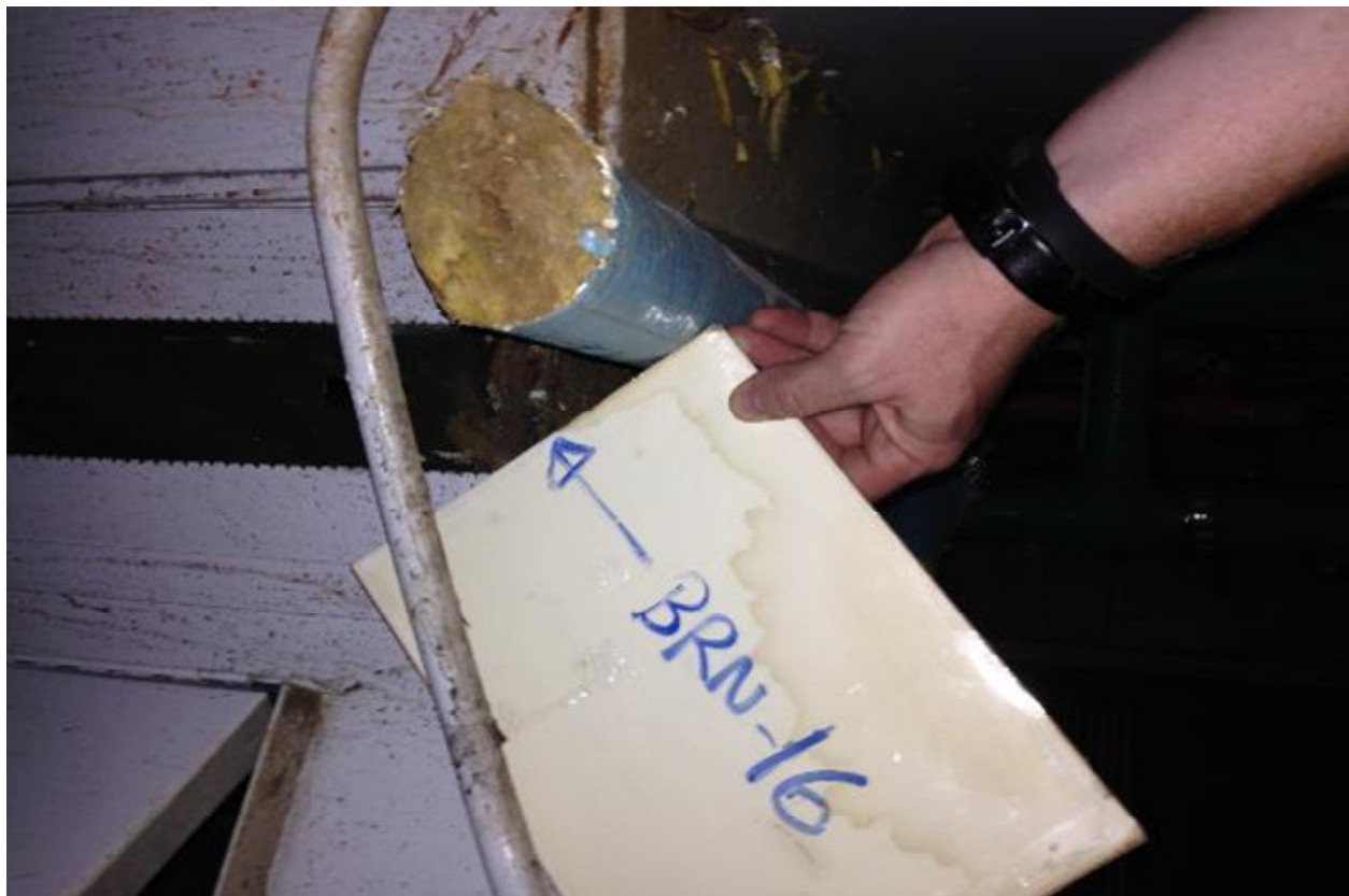
Plate 16: Laboratory analyses did not detect asbestos minerals within HVAC gasket sample BRN-16 collected from the North Administrative Building mechanical room.
