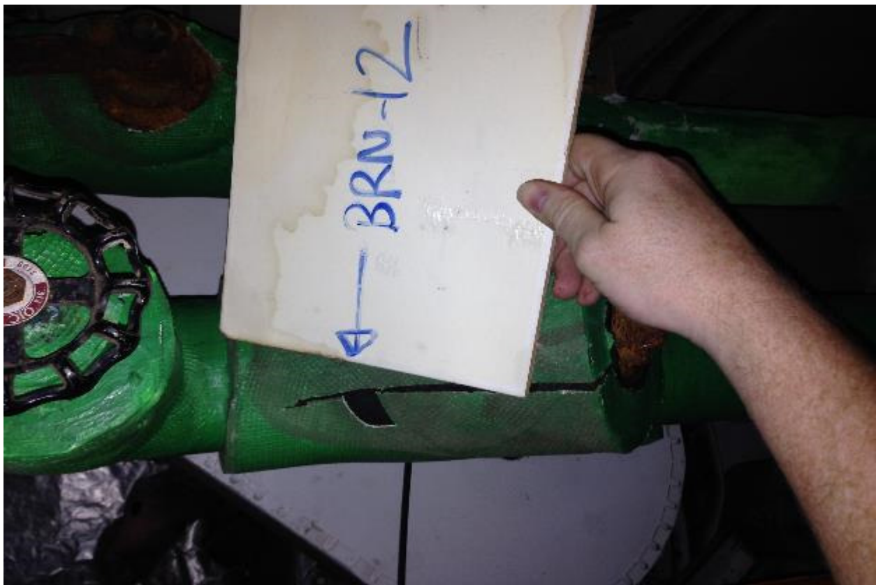
Plate 12: Laboratory analyses did not detect asbestos minerals within plumbing insulation sample BRN-12 collected from the North Administrative Building mechanical room.
