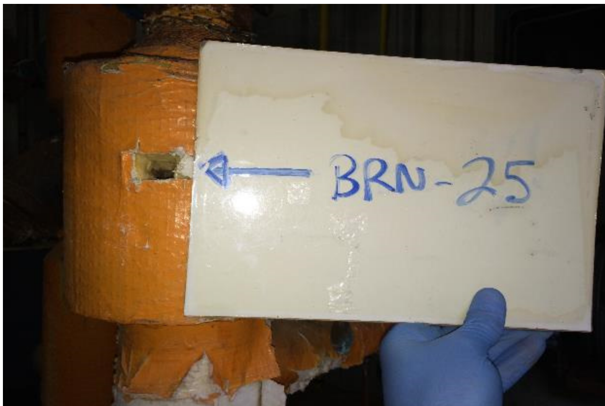
Plate 25: Laboratory analyses did not detect asbestos minerals within plumbing insulation sample BRN-25 collected from the South Administrative Building outdoor mechanical room.
