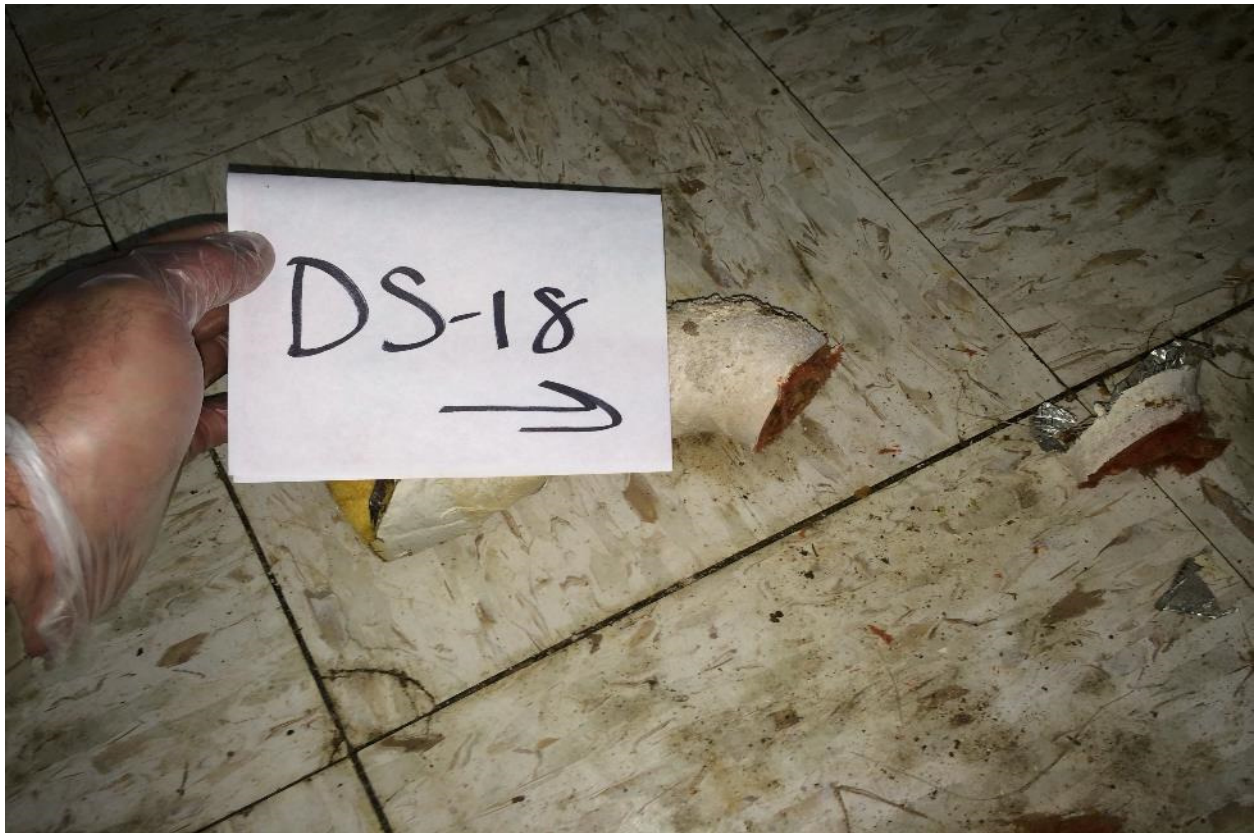
Plate 43: Laboratory analyses did not detect asbestos minerals within plumbing insulation sample DS-18 collected from the Dormitory Building downstairs training room.
