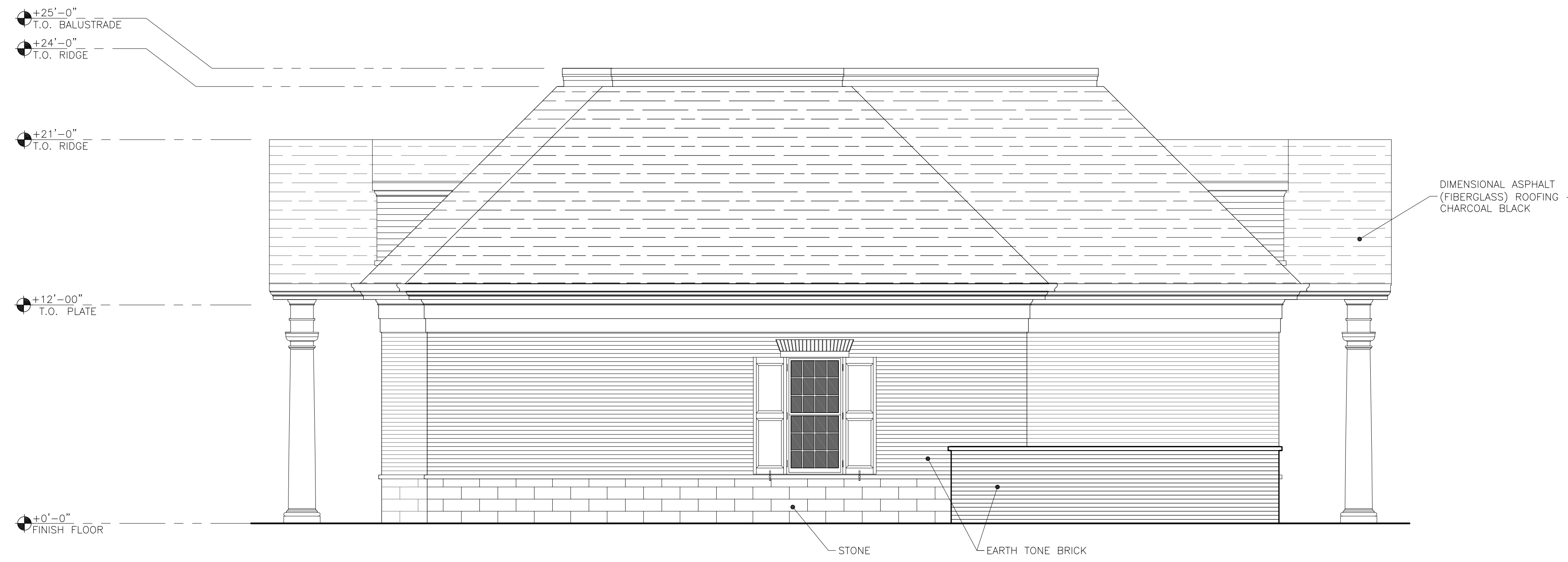
NORTH ELEVATION SCALE: 1/4" = 1'-0"
