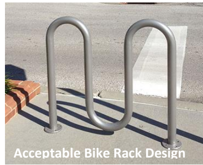
Figure 12-1A: Acceptable Bike Rack Designs
