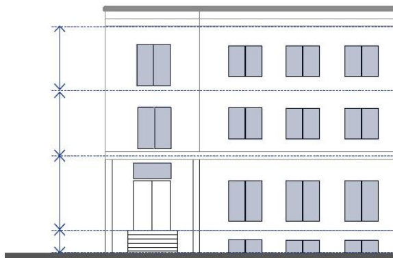
Figure 27-107D-4 Measuring Fenestration per Façade
