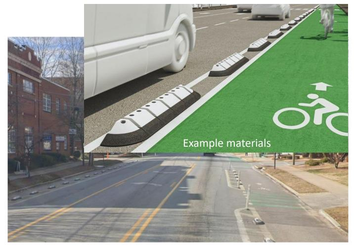
Alternate configuration – combination of flex posts and rubber markers
