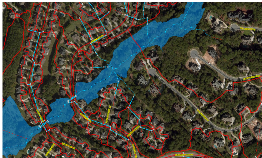
FIGURE 1: Dewberry created the Stormwater System Assessment Program for Gwinnett County, which is a watershed-wide H&H analysis that determines the existing pipe capacity level of service (LOS) of each County-maintained pipe throughout Gwinnett County. Dewberry has also developed a cost estimation and Capital Improvement Project management tool that interfaces with the stormwater database which assists the County with project and cost planning.
