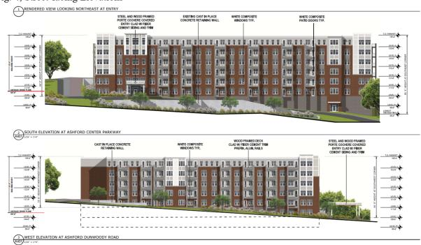
The applicant proposes a six-story residential building above a parking structure with a maximum height of 95 feet. The street-facing elevations will be clad in a mixture of earth-toned brick and fiber cement siding.
